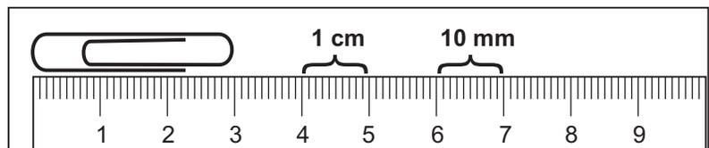
Fig. 1-1 Centimeter Ruler (To Scale)
